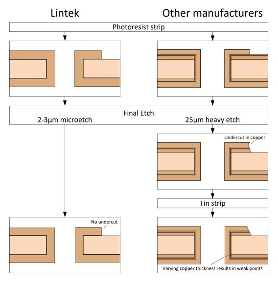
In the standard process, the variation in copper thickness between the barrel plating and the surface can produce weakness in the corners of plated through holes. Since Lintek's process maintains uniform plating on all surfaces of the panel, the plated through holes are more reliable under a range of conditions.
