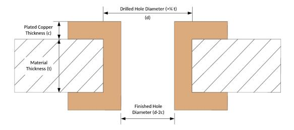
Using Lintek's vacuum copper deposition and additive technology, Lintek is able to produce plated vias with a standard finished hole aspect ratio of 5.3:1. Using our standard additive process, the drilling diameter of any plated through hole must be greater than ¼ the thickness of the layer/s it passes through.
