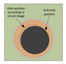
Finished hole size tolerances are as agreed between user and supplier. If no tolerance is specified, Lintek maintains default tolerances as shown on the table below.
