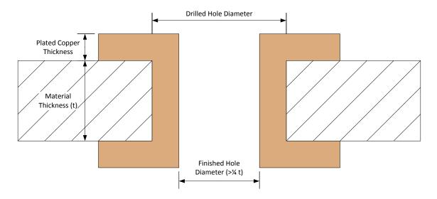
Lintek is able to produce plated vias with a standard aspect ratio of 4:1. As such, the drilling diameter of any plated through hole must be greater than ¼ the thickness of the layer/s it passes through.
